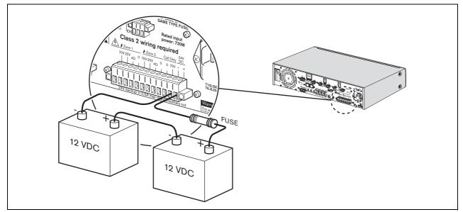
figure 4.1: Connecting a DC power supply
